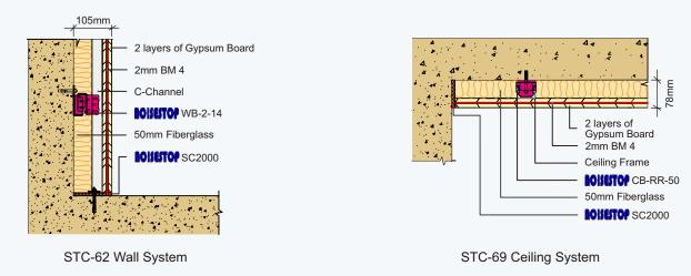
The normal way to increase the sound insulation of wall and ceiling is to increase the surface density of structure. BM 4 is an economical solution with only 2mm thick and very space saving for good sound insulation.
